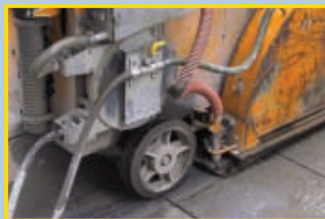
Watson-Marlow Bredel peristaltic pumps are used wherever quality and reliability are paramount – as here, powering coolant flow in a concrete-cutting machine in Japan. The pump is beneath the circular housing, center
